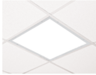
0078/1810/Q Recessed Ceiling LED 37W, 230V, 5000K, Lm3724, Size: 595*595*55mm Insulation Class I, IP40
