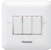
WBC5031 10A Plate Switch 3G, 1-Way SP 10AX 250V~
