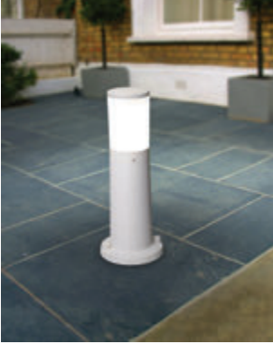
AMELIA 400 Model No. DR2.574.E27 Moulded Color: ●Black ○ White Diffuser PMMA: ○Opal Size: H=400 x W=155 Insulation Class II, IP55
